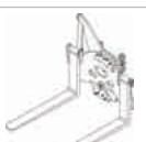
Rotators are used in various industries from waste management to poultry. This attachment allows flexibility in emptying containers offering a variety of features or angles of rotation from 50° to 360°.
