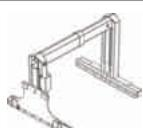
Block Grabs are used in the brick and block industries to handle a variety of pallet-less products.
