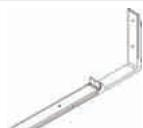
Reach forks allow one side off loading; this type of fork can extend outward to lift the load from the far side of the trailer bed. Reach forks provide up to an extra meter and consists of a standard fork with a second extendable fork.
