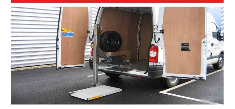
This lightweight and quick fit lift is easy to use and when not in use, simply sits to one side allowing unrestricted access to the rest of the vehicle. This lift can be fitted behind the rear or side door.
