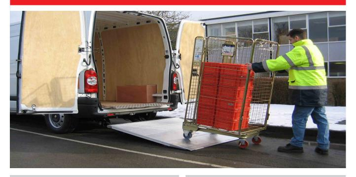
Developed for factory panel vans, this lift comes with a 1300mm deep platform, as standard. Use of high quality materials minimizes installed weight thus optimising vehicle payload.
