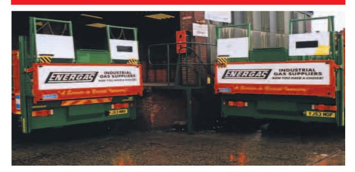
This robust column tail lift has been designed to suit the gas bottle market. As standard, the lift is installed with a pair of auto erect guards to ensure maximum operator protection at all times. We also include security chains with the lift which allows the operator to securely strap all bottle in position.
